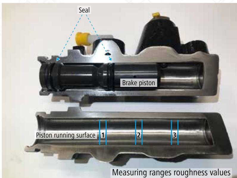
Figure 3: Interior view of the cylinder. Ranges of measurements for the roughness values on the functional surfaces of the two piston seals.
