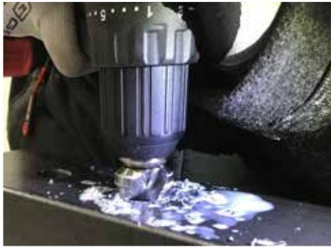
Figure 5: Drilling test The BLACK EDITION cordless drill made a hole up to 26mm in diameter. The market competitor drilled a diameter of up to 20mm.
